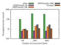
Fig. 5: Comparison of the throughput of ePipe/HopsFS, HDFS INotify, and Trumpet. HDFS INotify clients can set the maximum number of events to request from the namenode, so we compare against three different configurations for HDFS INotify (1K, 10K, and 100K). The default and recommended configuration for HDFS INotify is 1K. The Y-axis is in log scale with base 10.
